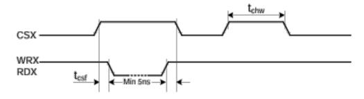
8. The Write to Read or the Read to Write timing:
