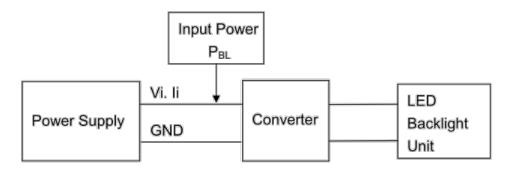
Note 3: The "LED life time" is defined as the module brightness decrease to 50% original brightness at Ta=25°C and If =120mA. The LED lifetime could be decreased if operating If is larger than 120mA. Note 4: LED light bar circuit:
