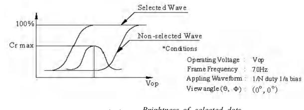
$$Contrast \ ratio(Cr) = \frac{Brightness \ of \ selected \ dots}{Brightness \ of \ non-selected \ dots}$$
